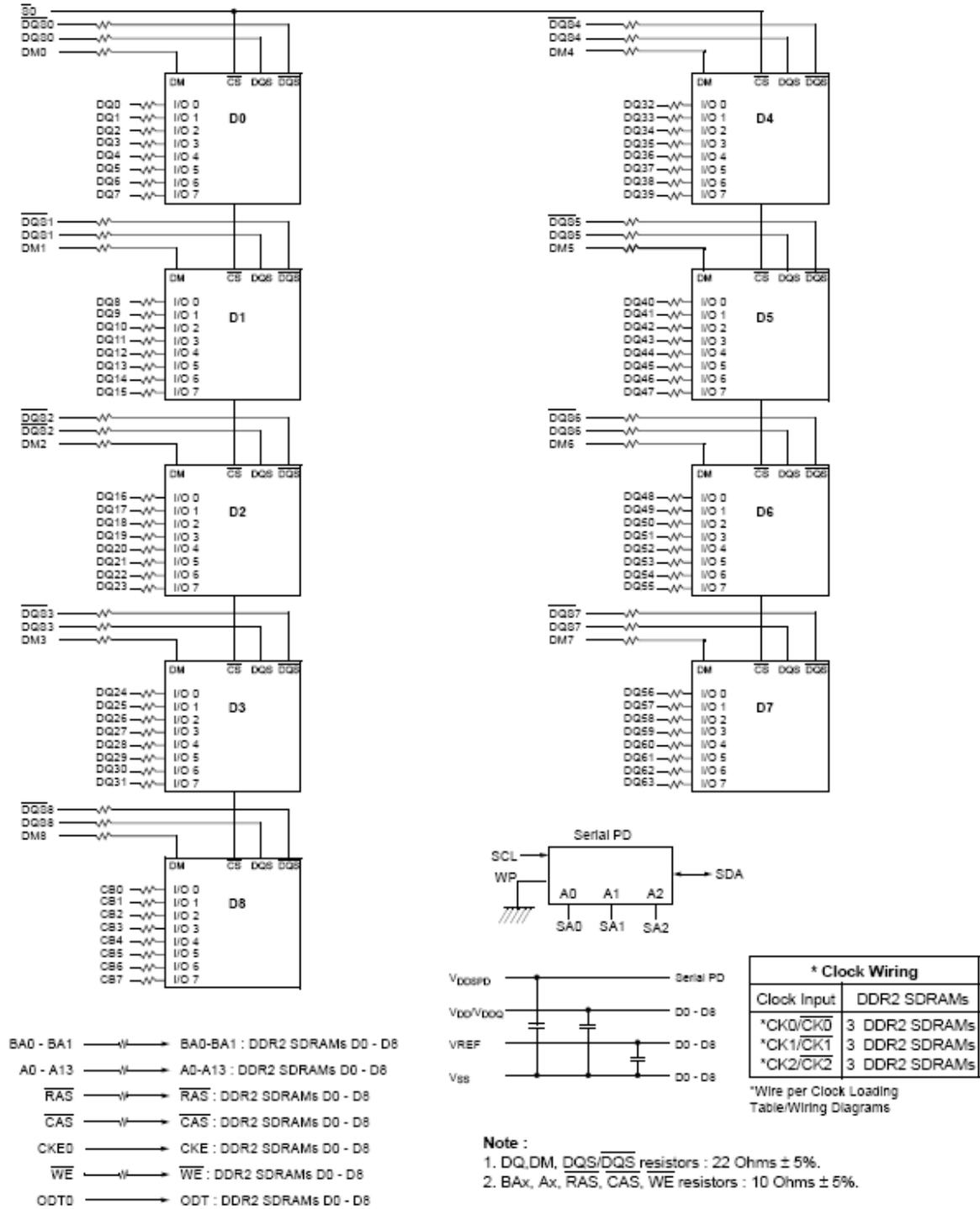
**FUNCTIONAL BLOCK DIAGRAM (GR2DD8B-E512XXX)**
